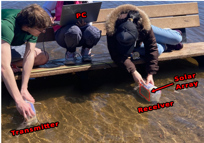
Fig. 5: Experimental setup for daytime testing in the Keweenaw Waterway, replicating the laboratory configuration. Both solar panel and laser were submerged, and the laser was manually aligned to illuminate the center of the solar panel receiver at a distance of 1 m. The receiver enclosure received power via connection to a PC using a USB serial interface, while the transmitter operated independently on battery power.
